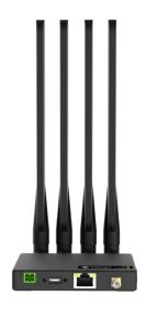
UF31 is a high-performance 5G modem for 5G wireless networking applications. It supports 5G NSA&SA, 4G LTE and 3G networks from telecom service providers of most countries in the world. The USB type-C port and Ethernet port are adopted to provide high-speed internet access for field devices.
