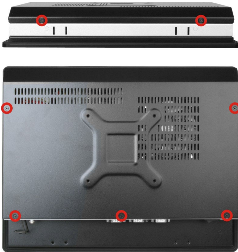
Figure 3-1: PPC-F15A-H81 Back Cover Retention Screws
