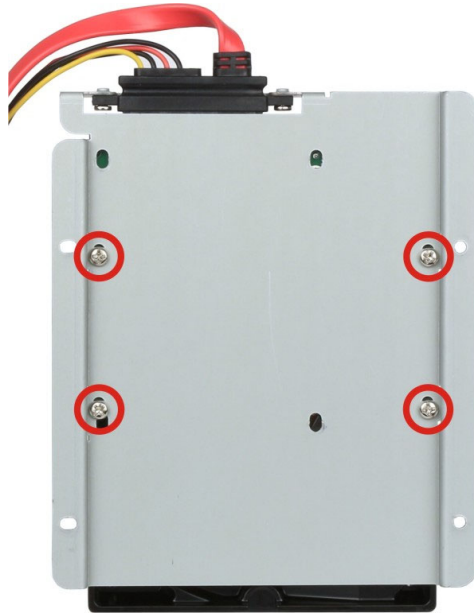
Figure 3-10: 3.5" HDD Retention Screws
