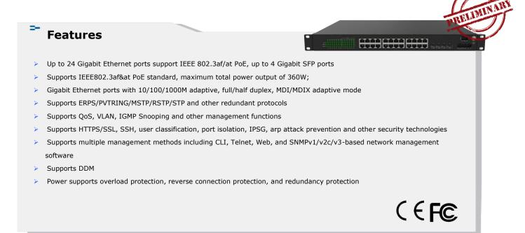
RGPS-3244GP-P is layer2 managed Ethernet switch with 24 PoE ports. The switch support Ethernet Redundancy protocol, MSTP (RSTP/STP compatible) can protect your mission-critical applications from network interruptions or temporary malfunctions with its fast recovery technology. And support wide operating temperature from -40 °C to 75 °C.
