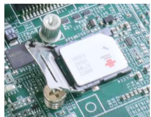
Push the SIM holder in the direction shown Flip open the holder and place SIM
