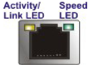
Figure 3-12: RJ-45 Ethernet Connector
