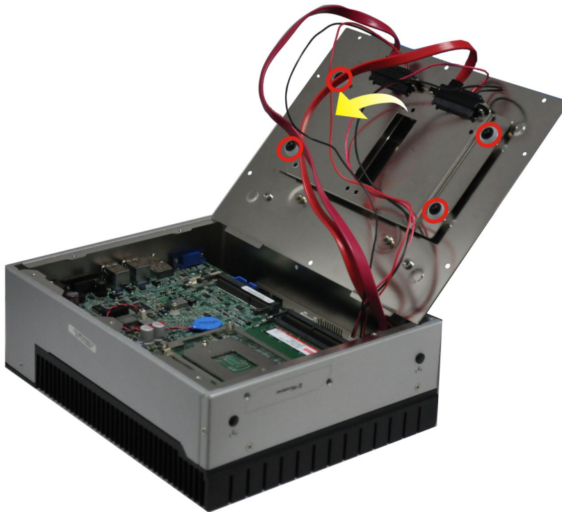
Figure 3-2: HDD Bracket Retention Screws
