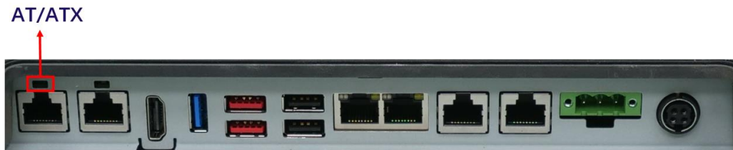
Figure 3-4: AT/ATX Switch Location
