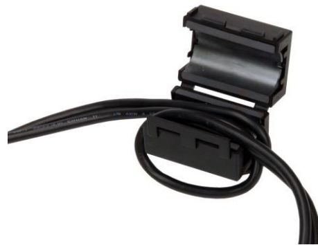
Figure 3-6: Wrapping Cable around the Core
