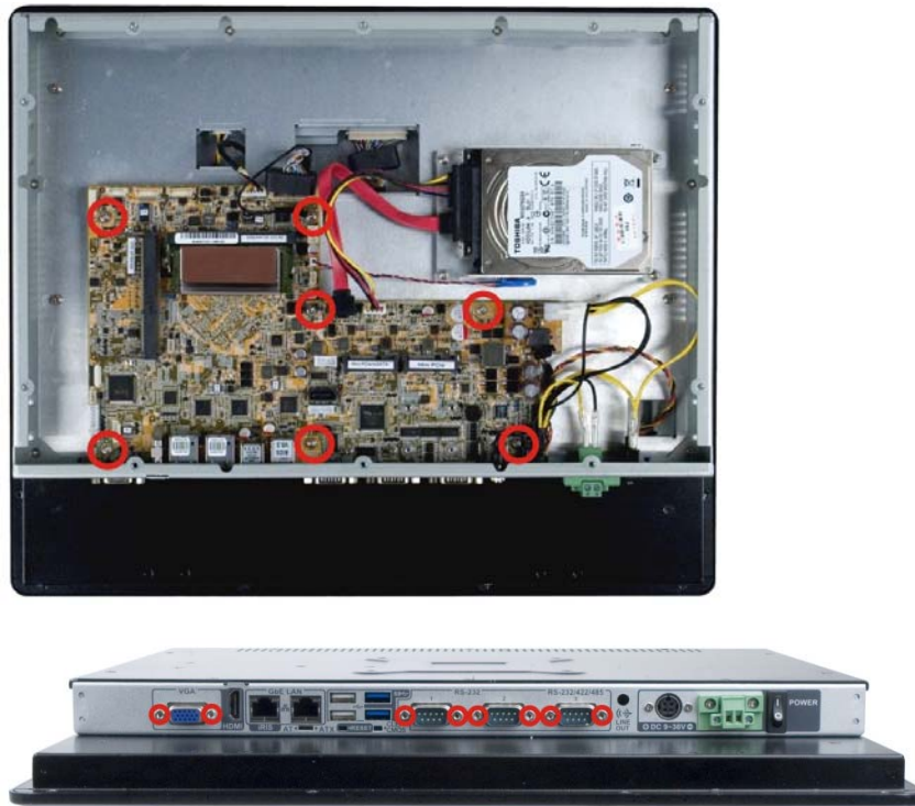
Figure 3-12: Motherboard Retention Screws
