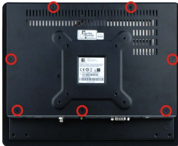
Figure 3-2: PPC-F10B-BT Back Cover Retention Screws
