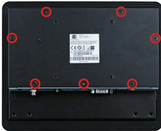
Figure 3-1: PPC-F08B-BT Back Cover Retention Screws
