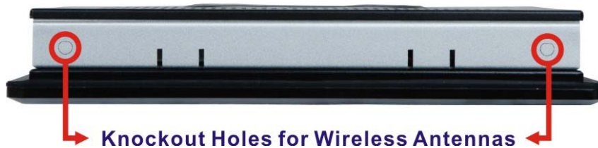
Figure 3-8: Knockouts on Top Panel for Wireless Antennas
