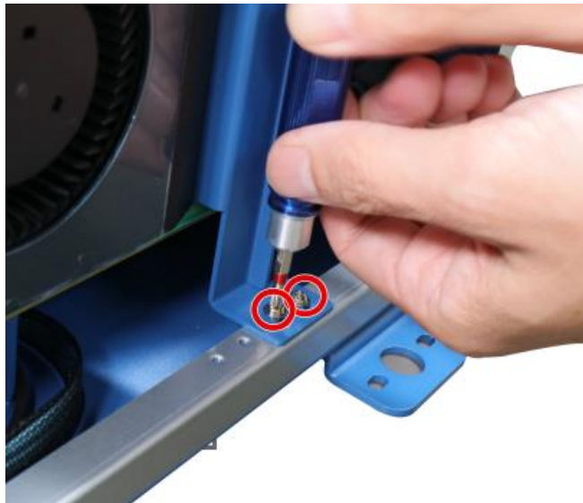
Secure bracket to the bottom of the enclosure
