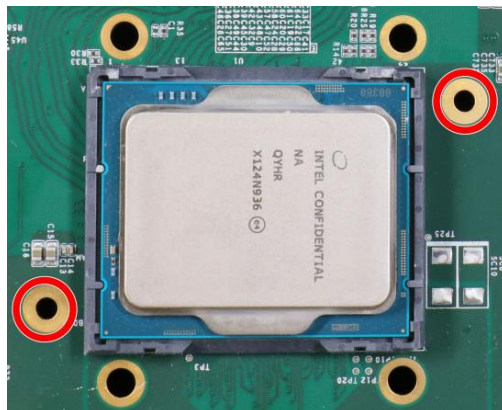
Screw holes for CPU retention bracket
