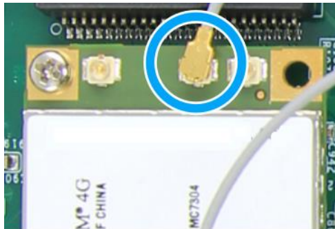
Clip on IPEX-to-SMA cable
