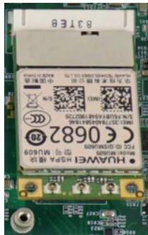
Insert on 45 degree angle
