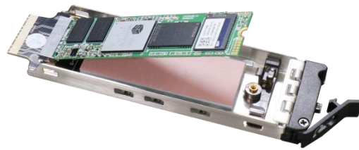
Insert on a 45° angle
