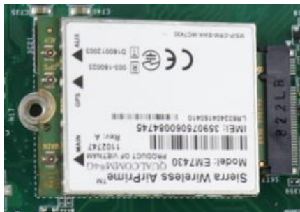
Insert on 45 degree angle
