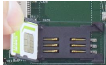
Insert SIM card with pins facing up
