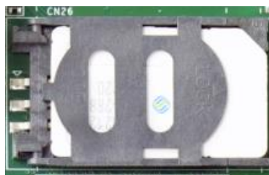
Slide and lift SIM card holder
