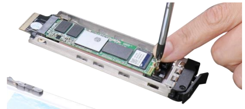
Secure with a screw
