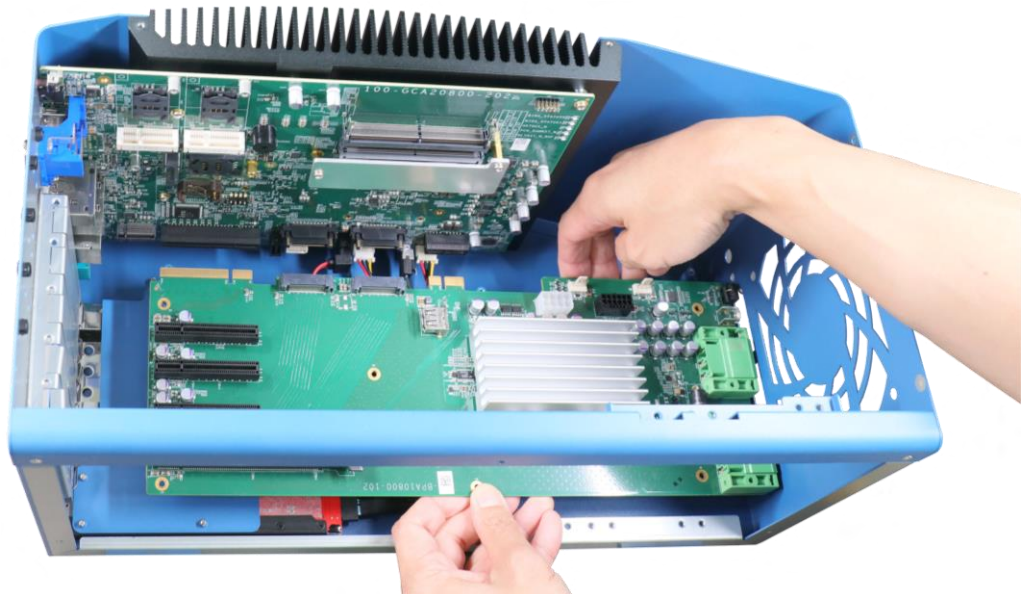
Disengage the daughterboard from the motherboard
