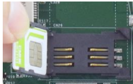
Insert SIM card with pins facing up
