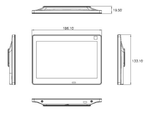
Figure 1-5: Physical Dimensions (millimeters)
