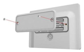
Figure 3-3: Battery Cover Reinstallation
