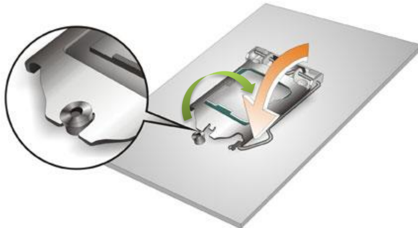
Figure 4-6: Close the Socket LGA1200
