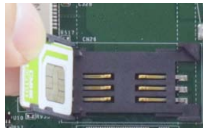
Insert Mini-SIM card with pins facing up
