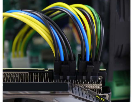
6 or 8/ 8-pin power connector on graphics card
