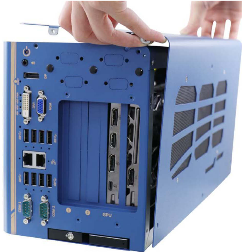
Place L-shape side panel onto the enclosure
