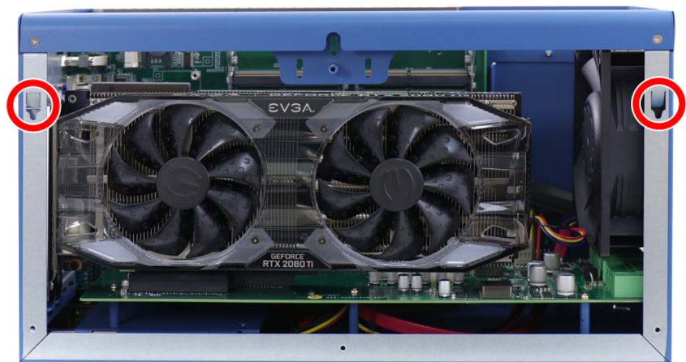
Slide-and-lock into the indicate hinges
