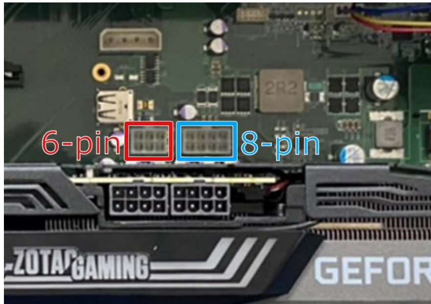
6/ 8-pin power connector on daughter board
