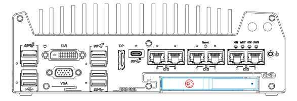
The Nuvo-9000LP series supports an external 2.5" HDD/ SSD via a hot-swappable slot. Designed for easy access, the HDD/ SSD slot is secured by a lock (indicated in **red**)and it supports RAID modes 0/1 configuration by combining with the internal HDD/ SSD drive for OS installation (coupled with the internal HDD). To set up RAID, please refer to RAID Volume Configuration section for details.
