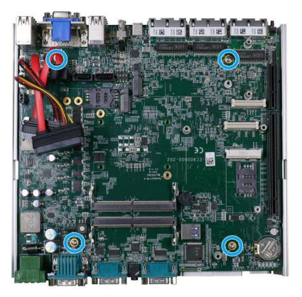
Secure motherboard with four screws
