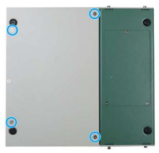
2. Gently wiggle the Cassette module and separate it from the system enclosure.
