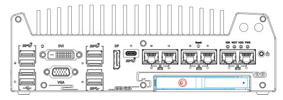
The system features a 2.5" external hot-swappable HDD/ SSD slot (indicated in blue), and secured by a lock (indicated in red). It coincides with the internal drive and can be configured into RAID 0 or 1 storage. To install HDD/ SSD into the 2.5" external hot-swappable slot, please refer to the following procedure:
