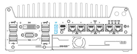
The system has a DisplayPort (DP) output which is a digital display interface that mainly connect video source and carry audio to a display device. When connecting a DP, it can deliver up to 4K UHD (4096 x 2304 @ 60Hz) in resolution. The system is designed to support passive DP adapter/ cable. You can connect to other display devices using DP-to-HDMI cable or DP-to-DVI cable.
