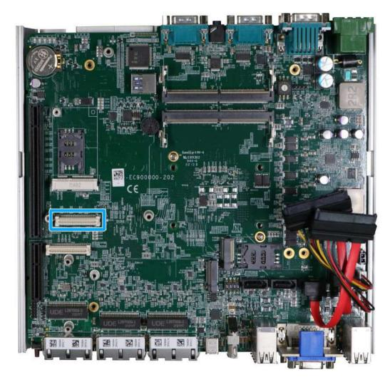
MezIO<sup>™</sup> is an innovative interface designed for integrating application-oriented I/O functions into an embedded system. It offers computer signals, power rails and control signals via a high-speed connector. MezIO<sup>™</sup> is also mechanically reliable benefited from its 3-point mounted mezzanine structure. A MezIO<sup>™</sup> module can leverage these signals to implement comprehensive I/O functions.
