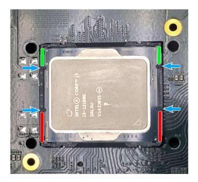
5. Locate the CPU retention bracket (holder) from the accessory box. Place the retention bracket on the CPU and hold it in place. Make sure the indicator triangle engraved on the CPU's integrated heat spreader (HIS) and the triangle indicator on the retention bracket are positioned in the same corner (indicated by blue circles).
