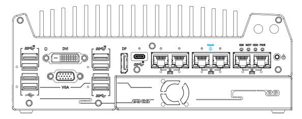
The reset button is used to manually reset the system in case of system halt or malfunction. To avoid unexpected reset, the button is purposely placed behind the panel. To reset, please use a pin-like object (eg. tip of a pen) to access the reset button
