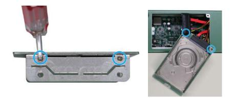
2 screws on each side per HDD/ SSD
