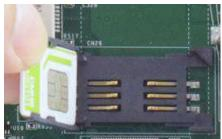
Insert Mini-SIM card with pins facing up
