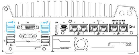
The system's USB 3.2 Gen2x1 ports (10Gbps) are implemented via native xHCI (eXtensible Host Controller Interface) controller and are backward compatible with USB3.2 Gen.1 USB 2.0, USB 1.1 and USB 1.0 devices. UFEI USB is also supported so you can use USB keyboard/mouse in UEFI shell environment. Indicated in **red** are screw-lock holes for the corresponding USB port.
