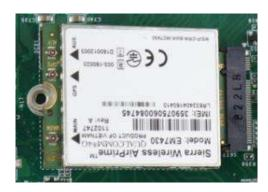
4. Gently press down and secure the module with an M2.5 P-head screw.
