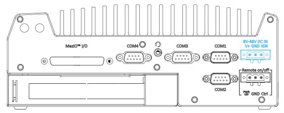
The system accepts a wide range of DC power input from 8 to 48V via a 3-pin pluggable terminal block, which is fit for field usage where DC power is usually provided. The screw clamping mechanism on the terminal block offers connection reliability when wiring DC power. In addition to DC power input, this terminal block can also accept ignition signal input (IGN) when ignition control module (eg. MezIO-V20) is installed for in-vehicle applications.
