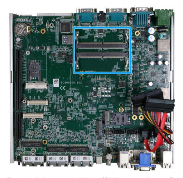
The system motherboard supports two DDR5 4800 SODIMMs memory module up to 64GB. Each slot supports single module SODIMM up to 32GB capacity.
