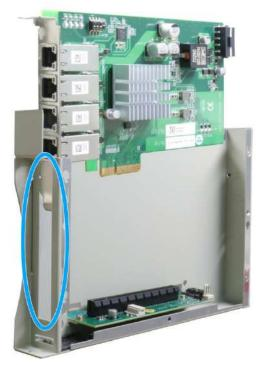
Remove bezel cover and insert the card
