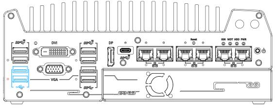
The USB2.0 ports are implemented via native xHCI (eXtensible Host Controller Interface) and are backward compatible with USB 1.1 and USB 1.0 devices. UEFI USB support is also provided so you can use USB keyboard/ mouse in UEFI shell environment. Indicated in **red** is a screw-lock hole for the corresponding USB port.
