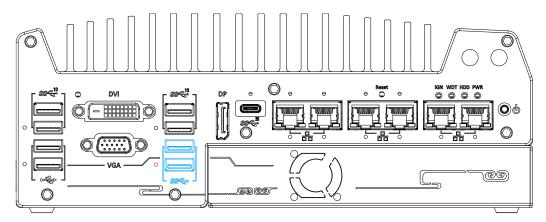
The system's USB 3.2 Gen1x1 ports (5Gbps) are implemented via native xHCI (eXtensible Host Controller Interface) controller and are backward compatible with USB 2.0, USB 1.1 and USB 1.0 devices. UEFI USB is also supported so you can use USB keyboard/mouse in UEFI shell environment. Indicated in **red** is a screw-lock hole for the corresponding USB port. xHCI driver is supported natively in Windows 10, therefore you do not need to install the xHCI driver prior to utilizing USB functions.
