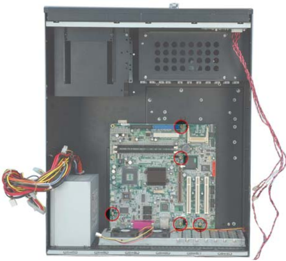
Figure 43: Motherboard Retention Screws
