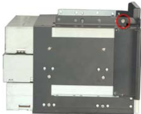
Figure 24: Top 3.5" Drive Bay Front Cover Retention Screws
