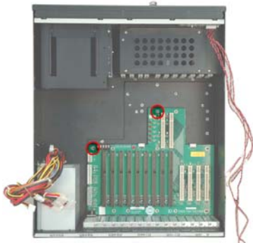
Figure 12: Copper Pillars in the Corresponding Holes in the Backplane
