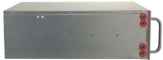
Figure 30: Front Handle Retention Screws
