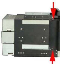
Figure 25: Left 3.5" Drive Bay Front Cover Retention Screws
