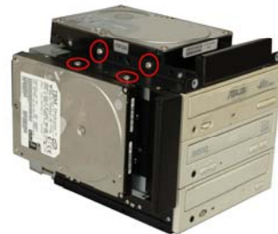
Figure 27: HDD Retention Screws
