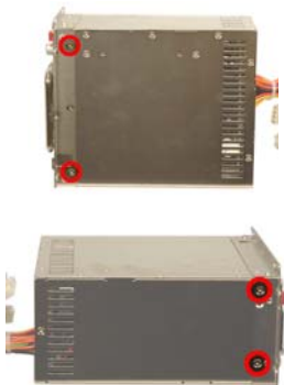
Figure 8: Redundant PSU Clamp Retention Screws
