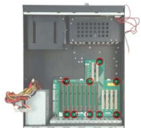
Figure 13: Backplane Retention Screws
