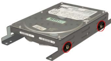
Figure 18: Internal HDD Clamp Retention Screws
