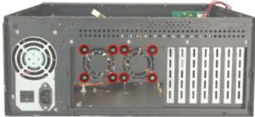
Figure 36: Fan Retention Screws
