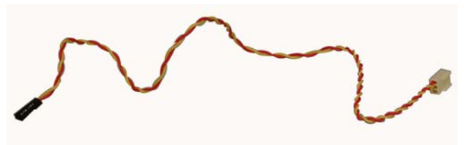
Figure 16: Backplane-to-CPU Card ATX Cable
