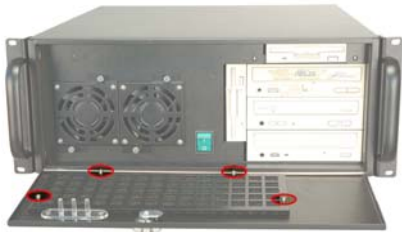
Figure 33: Fan Filter Bracket Retention Screws
