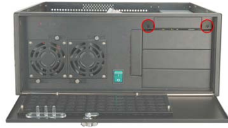
Figure 19: Drive Bracket Retention screws at the Front
