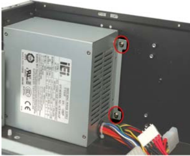
Figure 6: PSU Internal Retention Screws
