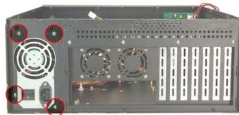
Figure 5: PSU Retention Screws at the Rear
