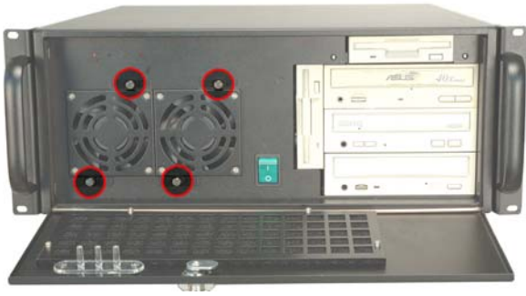
Figure 31: Fan Bracket Thumbscrews
