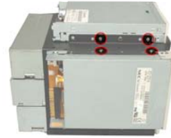
Figure 26: FDD Retention Screws
