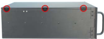
Figure 2: Top Cover Retention Screws
