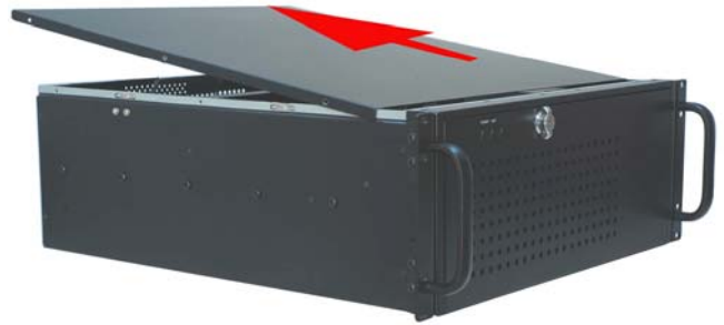
Figure 3: Remove the Top Cover
