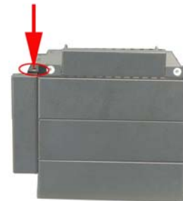
Figure 21: Left 3.5" Drive Bay Front Cover Retention Screws
