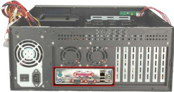
Figure 42: I/O Connectors installed in the I/O Connector Bracket
