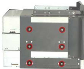
Figure 23: 5.25" Optical Drive Retention Screws
