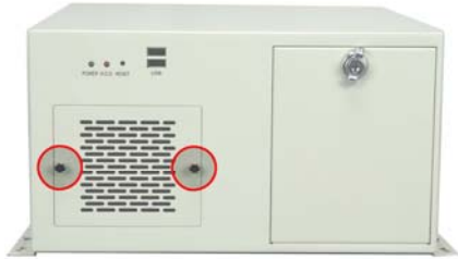
Figure 22: Fan Filter Bracket Thumbscrews
