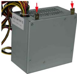
Figure 5: Slide Two Clip Nuts onto the Two Clips of PSU
