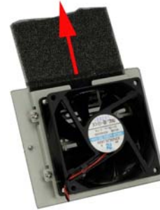
Figure 26: Pull the Fan Filter Pad Out
