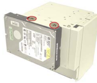
Figure 10: 3.5" Internal HDD Retention Screws
