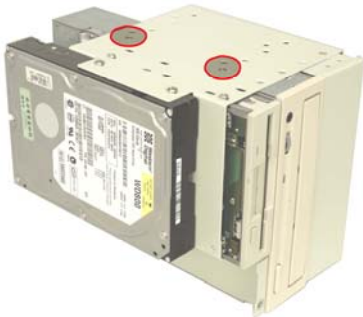
Figure 14: 5.25" Optical Drive Retention Screws
