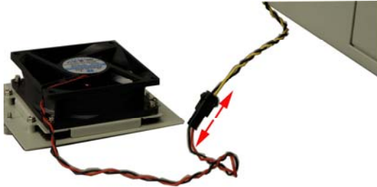
Figure 23: Unplug the Fan Power Cable
