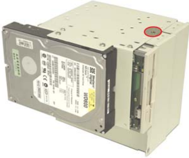
Figure 13: 5.25" Drive Bay Front Cover Retention Screws
