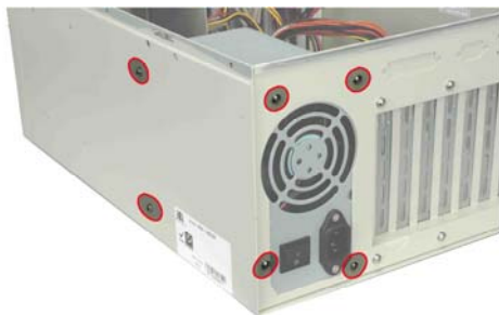
Figure 6: PSU Retention Screws
