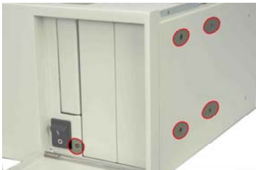
Figure 9: Drive Bracket Retention Screws
