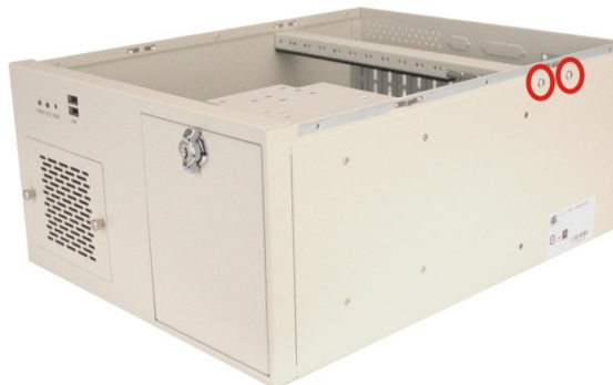
Figure 4: Remove the Hold-Down Clamp
