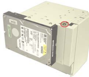
Figure 11: 3.5" Drive Bay Front Cover Retention Screws
