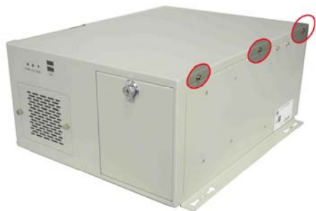
Figure 2: Top Cover Retention Screws
