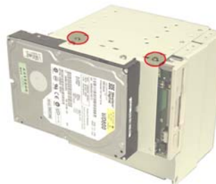
Figure 12: FDD Retention Screws
