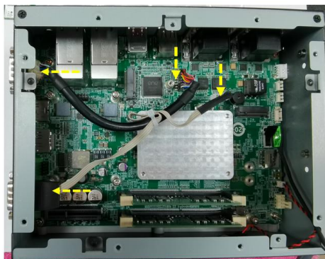
Figure 3-9: I/O Cable Installation
