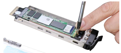
Secure with a screw
