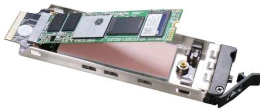
Insert on a 45° angle
