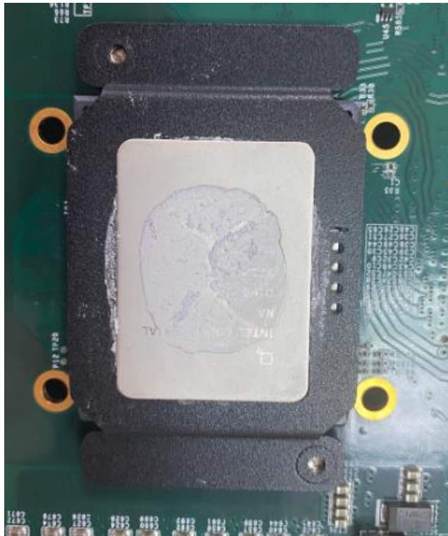
CPU retention bracket (holder)
