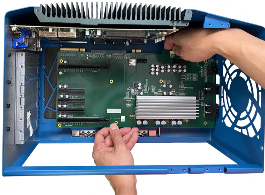
Disengage the daughter-board from the motherboard
