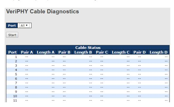
Press **Start** to run the diagnostics. This will take approximately 5 seconds. If all ports are selected, this can take approximately 15 seconds. When completed, the page refreshes automatically, and you can view the cable diagnostics results in the cable status table. Note that VeriPHY diagnostics is only accurate for cables 7 - 140 meters long.
