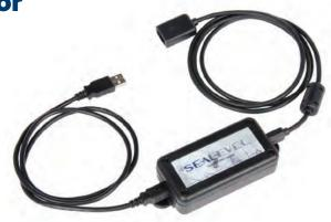
The ISO-1 is USB bus powered, eliminating the need for external power. The efficient DC/DC design allows energy transfer over the isolation barrier. The isolator provides up to 300 mA to a downstream USB device when connected to a standard 500 mA USB port. Additionally, the isolator can provide a full 500 mA to a downstream device when connected to a USB port capable of sourcing 1 A, or greater. Convenient high-retention USB connectors prevent accidental cable disconnections.
