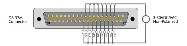
The diagram above diagram is representative of how lights (or other devices) can be controlled by the relay outputs. When relay 2 on the card is closed, it will allow current to flow from the power source, into pin 12 of the DB-37, through the optocoupler, out pin 30, and back to the power source thereby turning the light labeled "2" on.
