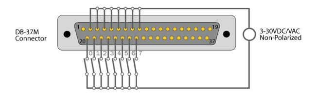
The diagram is representative of how dry contact inputs (or current / voltage sources) can be monitored by the optically isolated inputs. When switch 1 above is closed, it will allow current to flow from the power source, into pin 3 of the DB-37, through the optocoupler, out pin 21, and back to the power source. If the current flow is between 2 and 20 milliamps, this input will be read as logic "0". All the input associated with all open switches will be read as logic "1".
