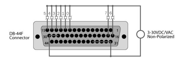
The above diagram is representative of how lights (or other devices) can be controlled by the relay outputs. When relay 2 on the card is closed, it will allow current to flow from the power source, into pin 12 of the DB-44, through the relay, out pin 30, and back to the power source thereby turning the light labeled "2" on.
