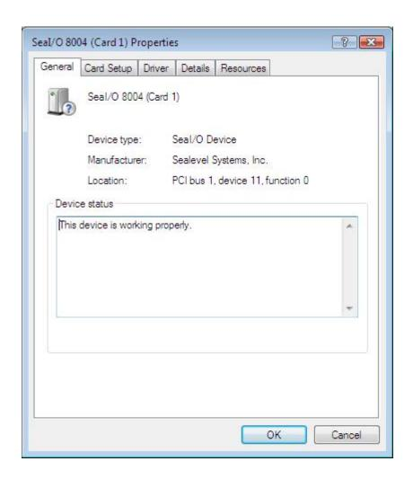
This verifies that the Seal/O digital I/O adapter (8004) is correctly enumerated.
