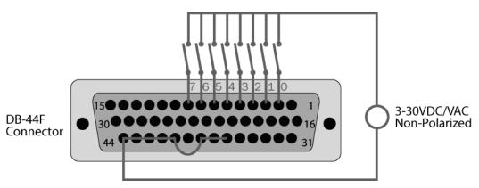
The above diagram is representative of how dry contact inputs (or current / voltage sources) can be monitored by the optically isolated inputs. When switch 1 above is closed, it will allow current to flow from the power source, into pin 3 of the DB-44, through the optocoupler, out pin 41, and back to the power source. If the current flow is between 2 and 20 mA, this input will be read as logic "0". All the input associated with all open switches will be read as logic "1".
