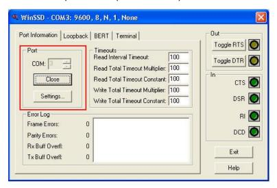
Click the 'Settings' button to open the COM Properties menu. Change your parameters to 9600 bits per second, 8 data bits, no parity, 1 stop bit, and no flow control, as pictured below.
