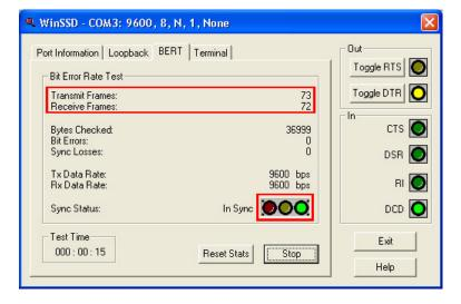
You can continue testing this port with different configurations or proceed with testing other ports, if necessary.
