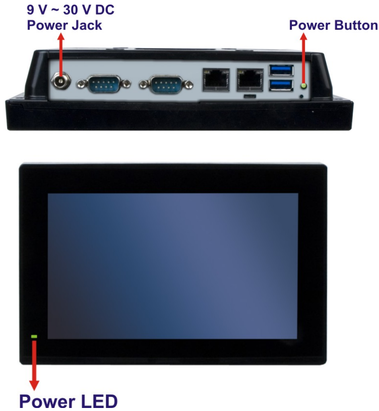
Figure 3-25: Powering On the System
