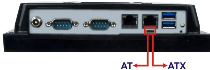
Figure 3-5: AT/ATX Switch Location
