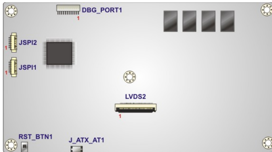
Figure 6-2: Main Board Layout Diagram (Solder Side)
