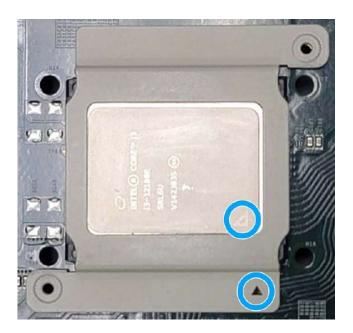
9. Turn the motherboard around and secure the bracket by tightening two M3 P-head screws.
