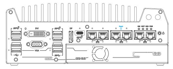
The reset button is used to manually reset the system in case of system halt or malfunction. To avoid unexpected reset, the button is purposely placed behind the panel. To reset, please use a pin-like object (eg. tip of a pen) to access the reset button
