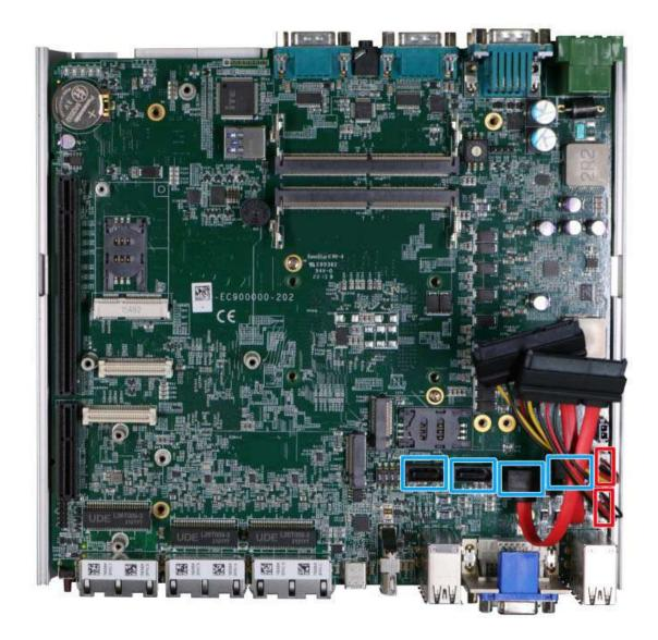
The system has four SATA ports which support Gen3, 6 Gb/s SATA signals. Each SATA port (indicated in blue) features a 7-pin SATA connector. However, due to mechanical restrictions, only two SATA ports can be accommodated inside the Nuvo-9000 series.
