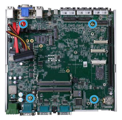
Secure motherboard with four screws
