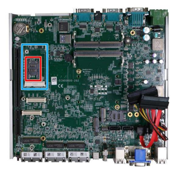
The system provides a mini-PCIe socket (indicated in blue) that is in compliance with mini-PCIe specification rev. 1.2. This mini-PCIe socket is designed with SIM card (slot indicated in red) support. With a SIM card installed, your system can access the internet via your network provider's 4G/3G network.
