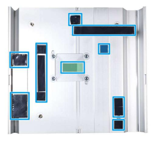
8. With the four motherboard standoffs aligned, gently lower the motherboard onto the heatsink and secure the four screws. Please remember to remove the protective film (indicated in red) on the CPU's thermal pad as well.
