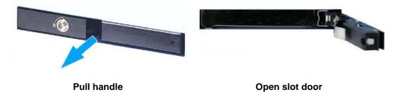
With the label side facing upward, insert the SATA connector side of the 2.5" HDD/ SSD into the slot first. You may feel resistance when the SATA connectors meet, push it firmly until the 2.5" HDD/ SSD is fully inserted into the slot.
