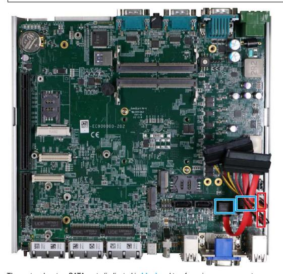
The system has two SATA ports (indicated in blue) and two four pin power connectors (indicated in red). The SATA and power cables should already be connected on the motherboard so users only need to install the HDD/ SSD. Please refer to the following instructions on how to install 2.5" SATA HDD/SSD.
