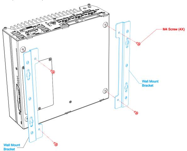
2. Place the system on a flat surface portion of the wall and secure it with four (4) M4 screws.
