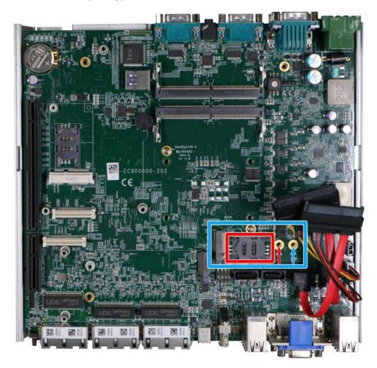
The system has an M.2 2242/ 3052 slot (indicated in **blue rectangle**) with a 5G/ 4G SIM slot (indicated in **red rectangle**). A copper standoff is provided for you to secure onto the motherboard into the **red arrow** location for an M.2 2242 module, or into the **blue arrow** location for an M.2 3052 module. By installing a 5G or 4G M.2 module and SIM card, you can access the internet via the provider's network.
