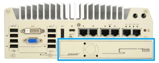
The Cassette module provides a separated compartment to accommodate add-on card(s). It compartmentalizes the heat generated and effectively manages thermal conditions of both the system and add-on card(s). The modular design reduces the complexity of installing and replacing add-on card(s) in the fanless controller. In addition, the mechanical design creates a sealed wind tunnel to bring in cold air and expels hot air via a system fan to offer the system extreme stability and reliability.
