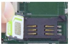
Insert Mini-SIM card with pins facing up
