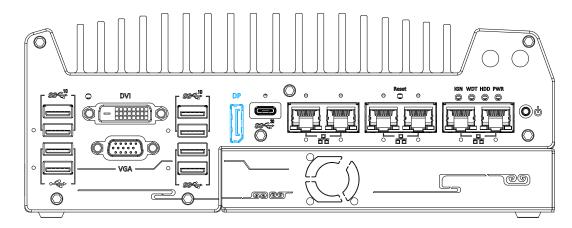
The system has a DisplayPort (DP) output which is a digital display interface that mainly connect video source and carry audio to a display device. When connecting a DP, it can deliver up to 4K UHD (4096 x 2304 @ 60Hz) in resolution. The system is designed to support passive DP adapter/ cable. You can connect to other display devices using DP-to-HDMI cable or DP-to-DVI cable.
