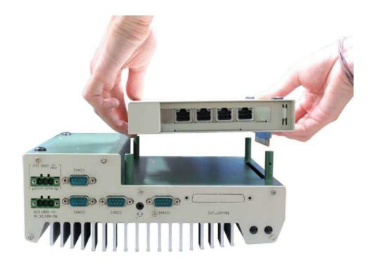
3. On the front I/O panel, remove the hexa-screws indicated below.
