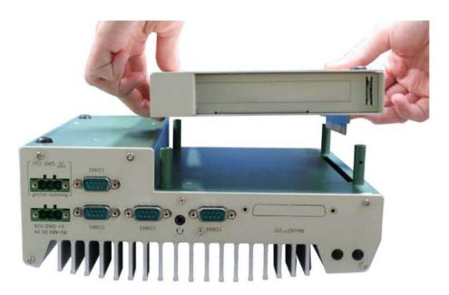
3. Remove the screw to open the Cassette cover.
