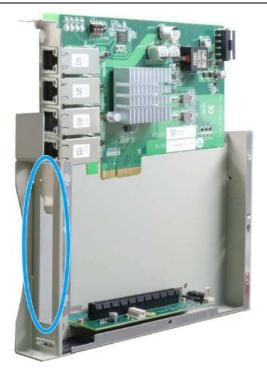
Remove bezel cover and insert the card
