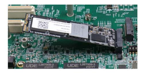
3. Gently press down and secure the module with an M2.5 P-head screw.
