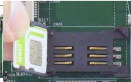
Insert SIM card with pins facing up
