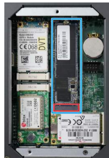
M.2 slot in red, SSD in blue
