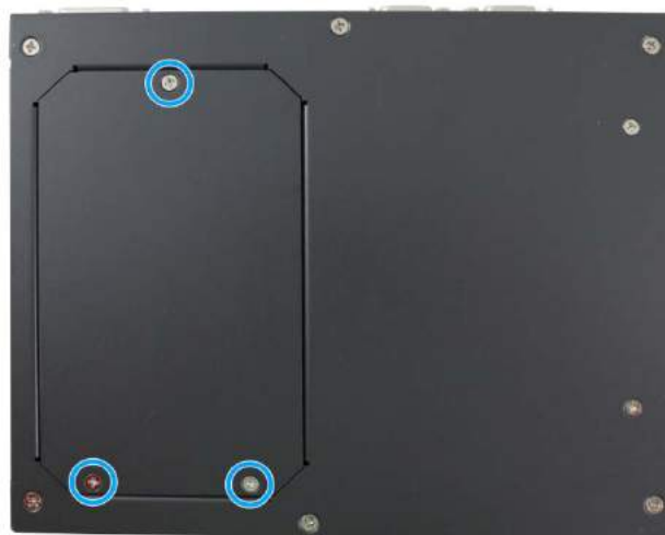
Remove screws indicated
