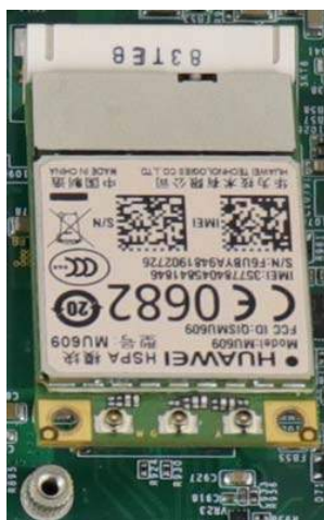
Insert on 45 degree angle
