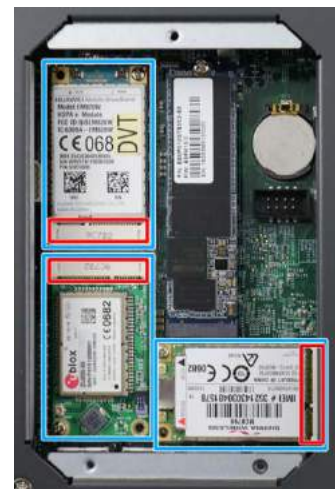
mini-PCle slot in red
