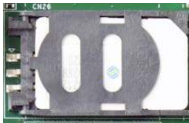
Slide and lift SIM card holder
