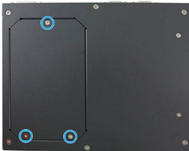
Remove screws indicated
