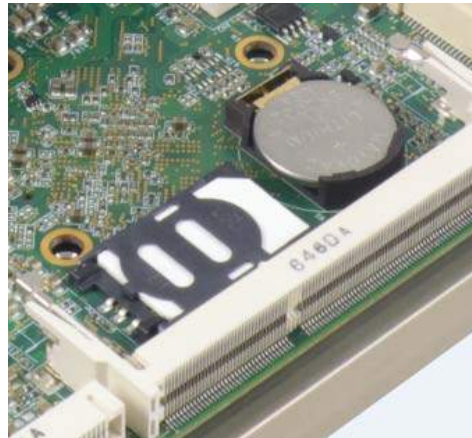
Secure the SIM card
