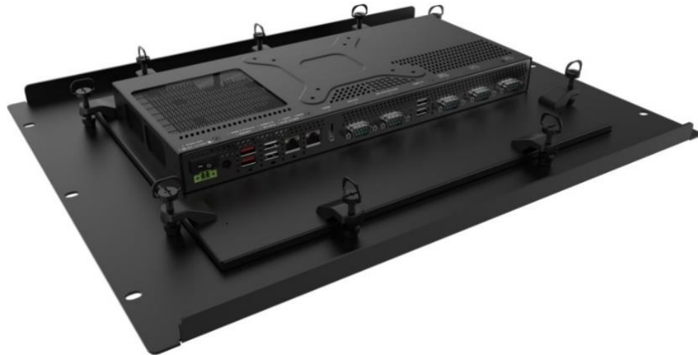
Figure 3-16: PPC2-xxx-ADLP Panel Mount Kit Installation
