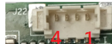
Figure 4: UART pin-out for Debug (J22)
