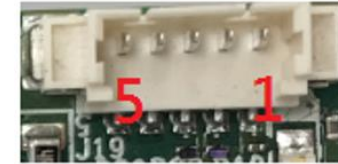
Figure 2: USB 2.0 Header for programming (J19)
