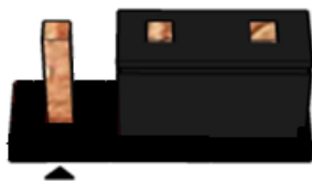
Pins 2&3: jumper position for VCC
