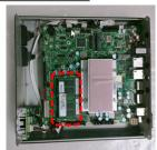
3. Install DIMM to MB on dash line area.
