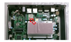
4. Install WiFi card on M.2 slot & plug in antenna IPEX header on WiFi card as arrow locations.
