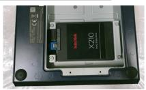
9. Install SSD to HDD bracket and install it to chassis.
