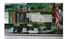
6. Install M.2 SSD on M.2 slot on dash line area.
