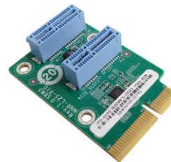
Figure 4-12: Outwards Riser Card Installation Example Figure 4-13: NWR-L2S-R10
