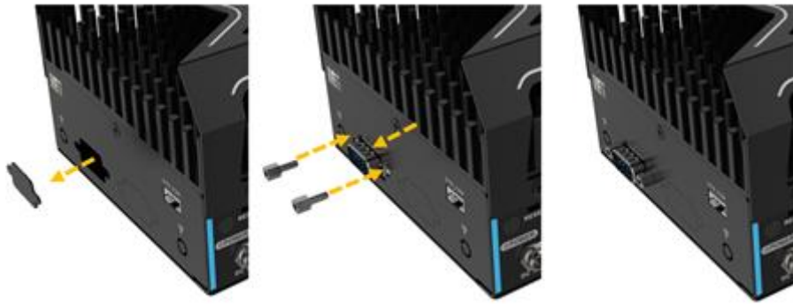
Figure 3-13: Knock out the reserved holes iDPM installation method
