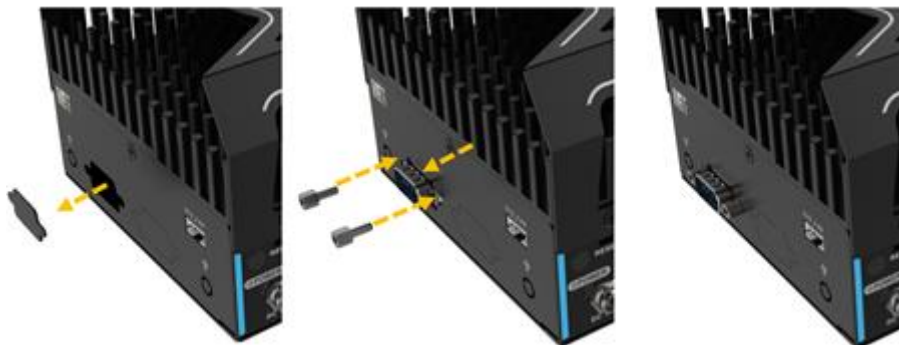
Figure 3-17: Knock out the reserved holes
