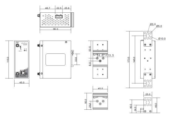
**IGAP-610+ Wall-mounting Measurements (Unit = mm)**
