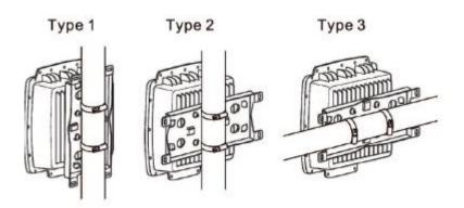
**IGAP-W612+ Pole-mounting Measurements**
