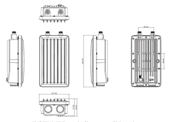
**IGAP-W612+ Wall-mounting Measurements (Unit = mm)**
