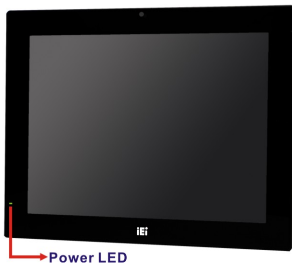
Figure 3-24: Powering On the System
