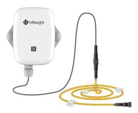
EM300-ZLD is a compact zone leakage detection sensor for detecting large area presence of water (or other liquids) and transmitting alarm using LoRaWAN® technology. With this low power consumption technology, EM300-ZLD can work up to 5 years with 4000 mAh battery. Combining with Milesight LoRaWAN® gateway and Milesight IoT Cloud solution, users can manage all sensor data remotely and visually and receive alarms via mobile APP.
