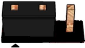
Pins 1&2: jumper position for 12V
