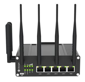
Adopting high-performance industrial platform of quad-core CPU and cellular module, UR75 is capable of providing wire-speed network and ultra-small package to ensure the extremely safe and reliable connection to the wireless network. Upgraded to the latest cellular technology - 5G, the UR75 makes itself possible to enjoy ultra-fast broadband access with 5G cellular network.
