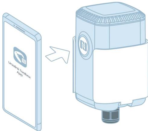
3. When you perform one of the following operations, enter the password and attach the smartphone with NFC area to the device until the APP shows a successful prompt.
