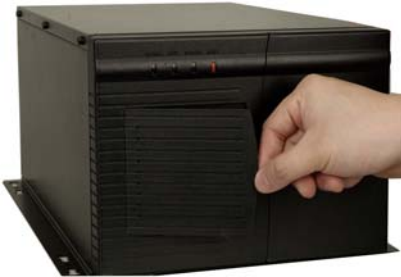
Figure 29: Flip Open the Fan Filter Cover
