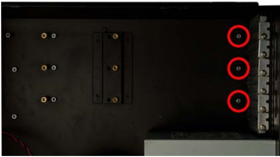
Figure 9: Three Predrilled Elevated Retention Screw Holes
