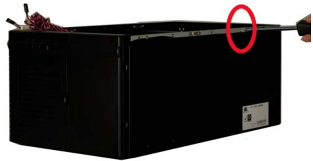
Figure 4: Remove Two Hold-Down Clamp Side Retention Screws
