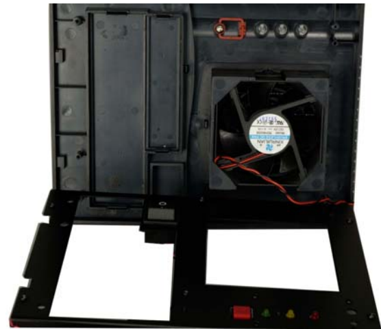
Figure 26: Remove the Metal Front Panel Plate
