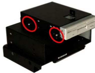
Figure 17: Secure a 3.5" FDD to the 3.5" Drive Bay
