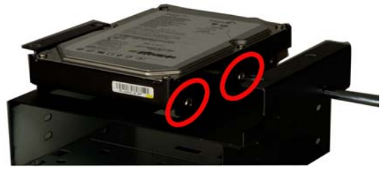
Figure 16: Secure an HDD to the Right Side of the Drive Bracket
