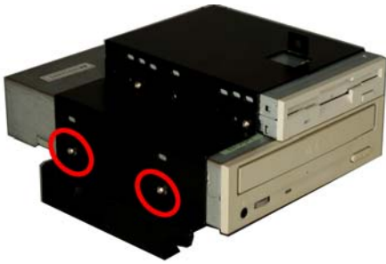
Figure 18: Secure a 5.25" Optical Drive to the 5.25" Drive Bay
