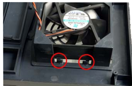
Figure 28: Two Fan Clips at the bottom of the Fan
