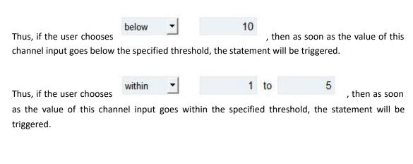
If you select a "Lockout Time" of 10s, a "Continue Time" of 5s, and choose above 10 , the statement will be triggered as soon as the value of the selected channel input goes above 10, and remains above 10 for 5s. It will then start checking the value of the selected channel input again after 10s and be triggered once more if the value of the selected analog input is above 10 for 5s.
