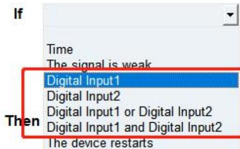
The user can setup multiple combinations; however, input 1 and input 2 must be activated before action is taken.
