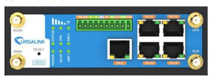
Locate the reset button on the router, and take corresponding actions based on the status of STATS LED.
