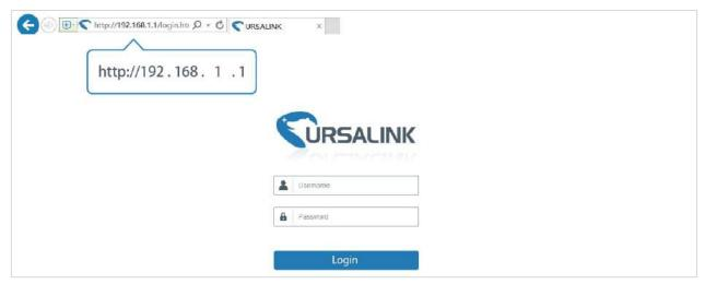
If the SIM card is connected to cellular network with public IP address, you can access WEB GUI remotely via the public IP address when remote access is enabled.
