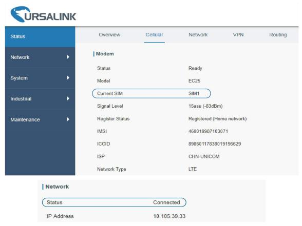
4. You can remove SIM1 to make the router fail to connect to network via it. Go to "Status > Cellular" again, and you will see the router is connected to the network through SIM2.
