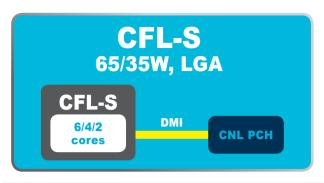
IEI PUZZLE-IN001 series adopts the New Xeon E & 8th Generation Intel® Core™ processor, of which the New Xeon E & core i7 is moving to six cores with Hyper Threading, Core i5 is moving to six cores, and Core i3 is moving to four core. The equipped LGA 1151 socket supports a wide range of performance options up to 65W TDP processors. There are two DDR4 DIMM slots are in PUZZLE-IN001 systems, and the memory capacity supports up to 32GB.
