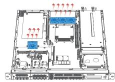
Users can define CPU fan and system fan speed and temperature profile in the BIOS menu. When the system is in idle or running less demanding tasks, smart fan is able to bring down the level of noise produced by rotating fans. The adjustable settings allow the PUZZLE-IN001 to be quieter during operation while extending the fan's lifespan, enhancing system stability and durability.
