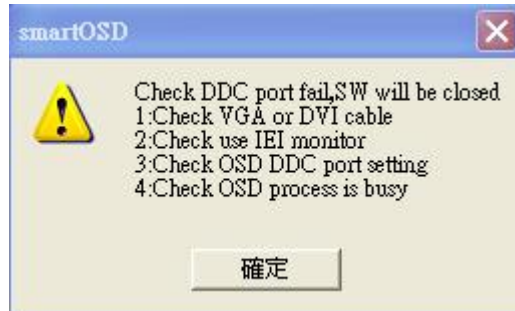
Figure C-18: DDC Port Failure
