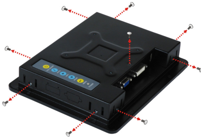
Figure 3-9: Rear Panel Retention Screw Removal (DM-F65A/08A)
