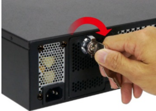
Figure 3-1: Unlock HDD Cover
