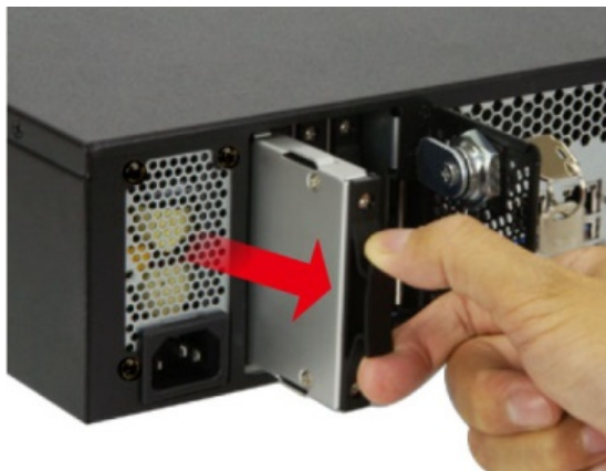
Figure 3-2: Drive Tray Removal
