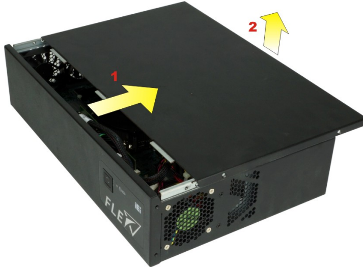
Figure 3-6: Remove the Top Cover
