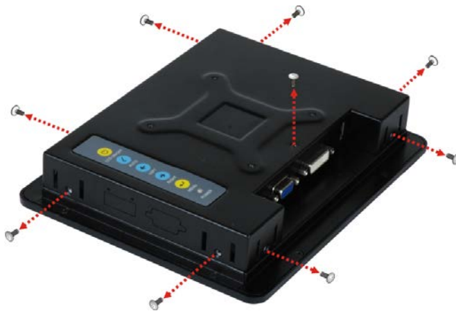
Figure 3-9: Rear Panel Retention Screw Removal (DM-F65A/08A)
