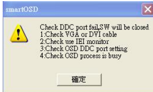
Figure C-18: DDC Port Failure
