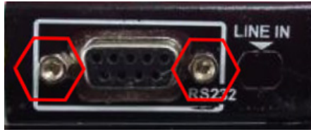
Figure 3-12: Hex Jack Screws for Securing RS-232 Connector
