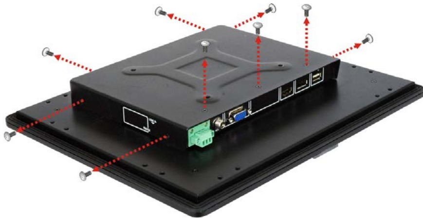
Figure 3-10: Rear Panel Retention Screw Removal (DM-F12A ~ DM-F24A)
