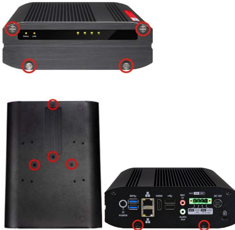
Figure 3-1: Bottom Panel Removal
