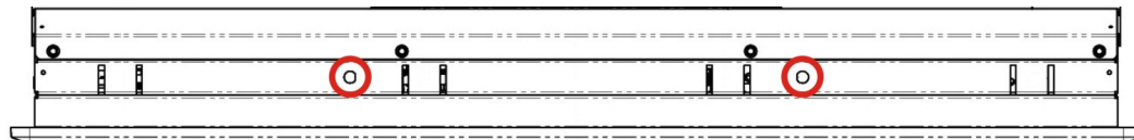
Figure 3-16: Knockouts for Wireless Antenna
