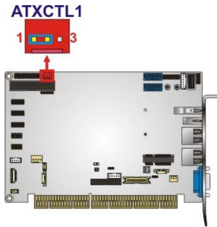
Figure 3-2: ATX Power Supply Enabled Connector Location
