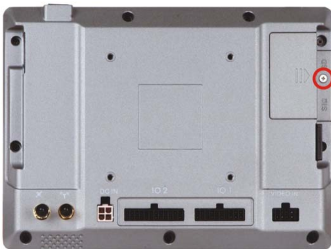
Figure 3-3: SIM Card Slot Access Panel Retention Screw
