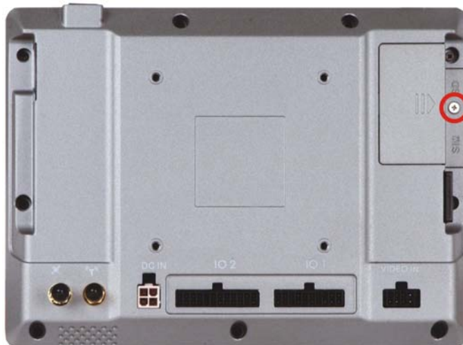
Figure 3-1: SD Card Slot Access Panel Retention Screw
