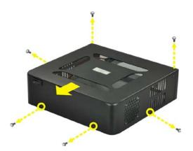
Figure 2: Top Cover Retention Screws
