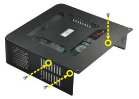
Figure 7: HDD Installation
