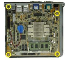
Figure 4: Motherboard Retention Screws
