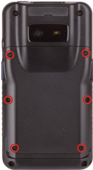
Figure 3-5: Battery Cover Retention Screws
